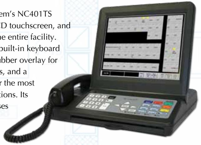
The Tek-CARE®400 P5 system integrates with a variety of ancillary systems. Pagers provide staff with a simple, cost-effective way to increase mobility and productivity—by sending calls to them almost instantaneously. The Tek-CARE®400 P5 system can also integrate with virtually any wireless telephone system, enabling two-way mobile communication between staff and patients.
